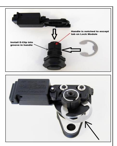
5) Reinstall the Emergency Handle and cables to the rotary latch, route the passenger side cable through the cable guide hole on the Lock Module the out to the rotary latch.
