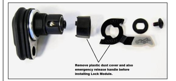
2) Locate and remove the black plastic Dust Cover if one is installed. May need to cut it off if necessary.
