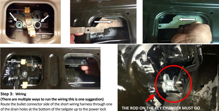
of the drain holes at the bottom of the tailgate up to the power lock assembly. Connect it to the bullet connectors of the power unit. Secure the wire with cable ties to prevent the wire from getting pinched or in the way of the latch rods. Connect the other end to the long wire THE ROD ON THE KEY CYLINDER MUST GO INSIDE OF THE LATCH FOR THE POWER LOCK
