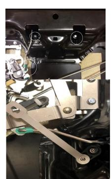
**STEP 2** - Remove the handle rod from mechanicals by turning the green rod clip and pulling the rod out of the clip. Swing the rod up and out of the way. Unplug the camera from the tailgate connector. Remove the two screws holding the factory handle in place; there are tabs that will hold the handle from falling out of the tailgate, but for extra assurance hold the handle in place so not let the handle to fall. Remove the factory handle.
