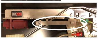
**STEP 6** – Replace the slide bolt that is on the power lock with the supplied crank link, screw, and washer as shown in the picture. Test functionality to ensure that everything is working properly.
