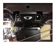
**STEP 2** - Remove the handle rod from mechanicals by turning the green rod clip and pulling the rod out of the clip. Swing the rod up and out of the way. Unplug the camera from the tailgate connector. Remove the two screws holding the factory handle in place; there are tabs that will hold the handle from falling out of the tailgate, but for extra assurance hold the handle in place so not let the handle to fall. Remove the factory handle.
