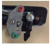
Remove the nut from the lock cylinder and remove the lock
