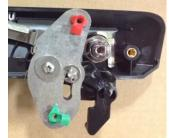
Remove the metal clip by sliding of the plastic lock adapter. Remove the plastic lock adapter by pushing it out of the bezel
