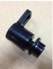
Install the cam/pawl assembly onto the back of the lock. The triangular opening must go around the post and the square cut out must align with the back of the square on the back of the lock cylinder. Put the washer on the screw and insert screw into the hole at the top of the cam/pawl assembly. Tighten screw tight.
