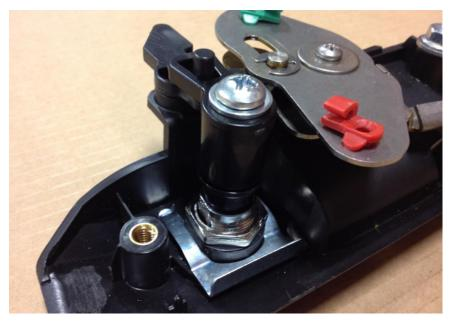
**Step 6:** If the lock operates properly, reinstall the handle into tailgate and reinstall the access panel.
