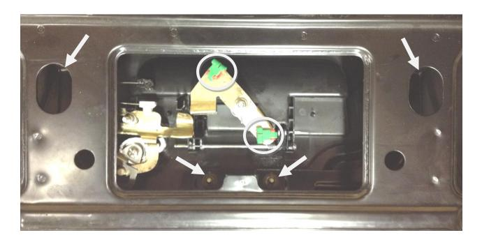
**Step 2:** Remove the latch rods from the plastic clips (circled on picture). Do this by prying up the top side of the clip and popping it open. Lift the rod out of the clip.
