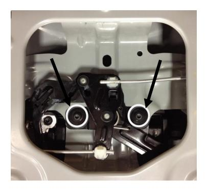
**Step 4:** - Shut the tailgate. Test the function of the lock. Turn the key counter clockwise to unlock. Turn the key clock wise to lock. If everything works reinstall the access panel.
