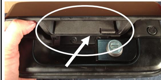
**Step 6:** Test the functionality of the lock by turning the key to the lock position and trying to lift the handle from the bezel. If prevents the handle from lifting away when locked reinstall the handle into the tailgate. Install the handle mounting bolts and tighten. Re-attach latch rods to clips. Install the access panel and bed liner if applicable.
