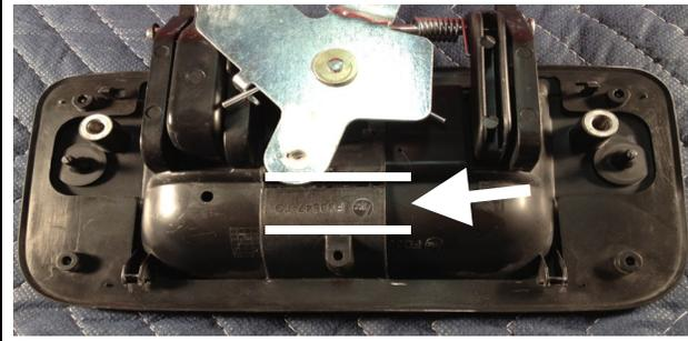
**Step 3:** Install the supplied support bracket as shown below using the factory bolts to hold the bracket in place. Using the holes in the bracket as a template drill through the plastic bezel using a 4mm drill bit. The arrows below point to the holes to be drilled.
