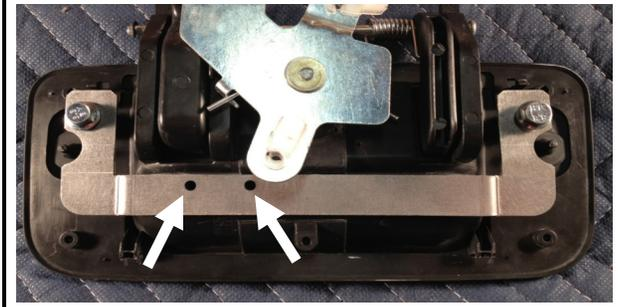
**Step 4:** Install the lock assembly from the **front** of the handle putting the threaded studs through 4mm holes that were just drilled (make sure the lock assemble is in the unlock position when installing). Install the 2-4mm washer and nuts on the studs and tighten. Now remove the factory mounting bolts that were used to temporarily hold the bracket in place.
