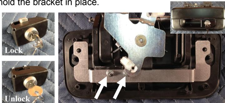
**Step 5:** Clean the area under the handle where the striker plate will be adhered with the provided alcohol wipe. Peel red backing of the 3M tape that is attached to the striker plate and install on the handle as shown below \*noting the slot and bend position, also the plate sits flush to bottom of the handle.
