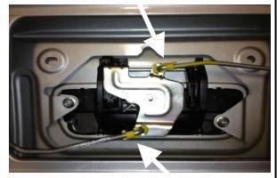
**Step 5**: Install the Pop & Lock into the tailgate in reverse (step 4-3-2) while making sure that it is in the locked position (fig. 1). Make sure that the bottom small tabs (fig 2) snap onto the tail- gate before tightening the bolts.
