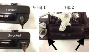
**Step 3**: Remove the handle mounting bolts from the factory handle.
