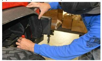
Apply masking tape to the Jeep body along the outside of the fender recess, to protect the paint while installing the Crusher Flare.
