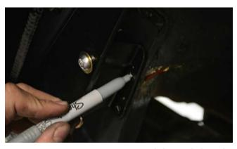
14. Use a fine-tip felt marker to mark the two holes to be drilled in the upper-rear corner, where the two remaining (non-countersunk) holes are, in order to install the Rear Inner Fender Bracket.
