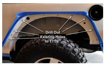
It is VERY IMPORTANT to be extremely careful when drilling these holes. Take extra care to ensure that the drill bit is exactly perpendicular to the sheetmetal, as it may "walk" and dislocate the resulting hole. Also be careful when drilling, as the thin sheetmetal may want to catch on the bit and deform it, making the subsequent nut-sert installation more difficult.
