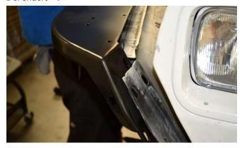
**24.** Use the OE hardware to bolt the DeFender™ to the firewall and to the grille. Leave the hardware somewhat loose until both DeFenders ™ are installed to this point in the instructions. On CJ's, the headlight bezel and assembly will need to be removed to access the top nut (this is the second hole down from the top, and not an original fender mounting hole which is now blocked by the new DeFender™).
