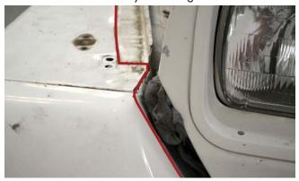
11. Cut along the traced cut-line with a pneumatic body saw, reciprocating saw, cut-off wheel or other appropriate cutting tool. Note that the sheetmetal is double thickness along the back portion of the fender. Also you will need to further loosen or remove the firewall bolts in order to pull the fender away from the firewall to continue your cut to the end.
