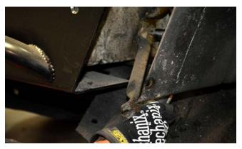
18. At this point your work should look somewhat like the photo below, with only the inner fender and a narrow strip along the top of the outer fender remaining. NOTE: your stock inner fender will NOT be attached to the Jeep's tub at this time—at this point in the installation process it will be unsupported except by the accessories bolted to it. This is normal. It will regain its rigidity once the DeFender™ has been installed.
