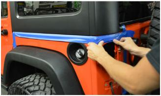
**10. Place the driver's side Crusher** Corner over the corner of the Jeep. The Crusher Corner will slip snugly over the fuel filler trim piece (and stock taillight housing, if present), assisting with aligning it. Use a measuring tape to ensure that the distance between the top edge of the Crusher Corner and the top edge of the Jeep's tub is the same from front to back, and securely clamp the Crusher Corner into place.
