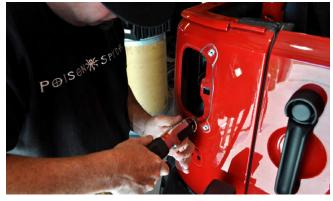
8. Use a file or sander to smooth the edges of the cut sheetmetal. It is important to remove any burrs or sharp edges which may snag, fray or cut electrical wires over time. Use some touch-up paint or clear-coat to seal the bare metal around the edge of the cut, to protect it from rust in the future.
