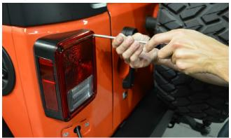
5. With your thumb, press on the release tab of the taillight harness plug, and separate it from the vehicle harness. Set the OE taillight assembly aside.
