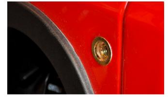
If you "spin" a nut-sert: That is, if it loses its grip due to over-tightening or improper installation, the quickest, easiest fix is to use a MIG welder to place a small tack weld at the edge of the nut-sert flange. Before applying the tack weld, sand or grind the paint from a very small area of the sheetmetal where the tack weld will be. Then insert a screw into the nut-sert to protect the threads from weld splatter. Only apply a very small tack or two, as you do not want to heat up and deform
