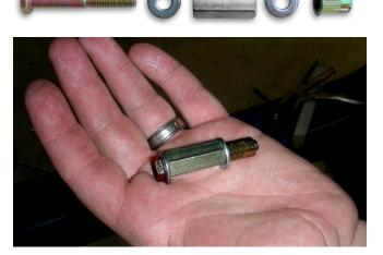
17. Use an open end wrench to hold the coupler nut stationary while turning the head of the bolt clockwise with a ratchet (or small impact wrench) and socket. As you turn the ratchet, the bolt will draw the far end of the nut-sert toward the inside of the sheet metal, gripping it with the knurled outside edge of the nut-sert as it deforms. Continue to turn the ratchet until the nut-sert is fully seated. DO NOT OVER-TIGHTEN as you can damage the nut-sert, or cause it to lose its grip.
