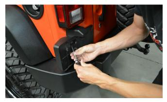
4. Use a Phillips screwdriver to remove the stock taillight assembly from the Jeep. Note that there are four screws, one in each corner of the taillight housing. You only need to remove the two inboard screws. Once these two screws are removed, grip the taillight assembly, slide it slightly toward the center of the Jeep and pop it out.
