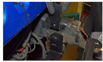
20. Insert a 1/2-13 X 1 Gr8 Hex Head Cap Screw with 1/2" Flat Washer through the corresponding hole in the side of the Recessed Winch Cradle, through the crash bar vertical support, into the Nut Plate. Leave this fastener loose.
