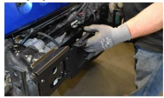
19. Insert a Nut Plate into the "crash bar" vertical support. Make sure the flush side of the nut plate is facing toward the center of the Jeep.
