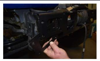
28. Note that the Spacer Plates are not symmetrical and must be oriented correctly, to match the four corresponding bolt holes in the Cradle and the frame. A spud bar or pry bar will be helpful in fine-tuning the placement of the spacer plate.
