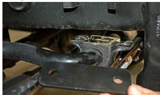
**14. Reinstall and re-tighten the two** swaybar bushing blocks.
