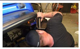
34. The best strategy is to first try to get one nut threaded on, on either side of the bumper, to start. Once there is at least one nut started on either side, it will be easier to coax the remaining threaded studs through their corresponding bolt holes.
