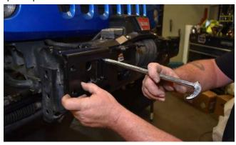
29. Pre-install a pair of LED cube lights (sold separately) into the light mounts of the Bruiser bumper. Use the mounting brackets that were supplied with the lights, to mount them to the light pedestals welded into the interior of the Bruiser bumper. Adjust the position of the light so that it is flush with the exterior surface of the bumper.
