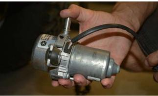
**10. Attach the vacuum pump into** the relocation bracket, oriented as shown in the photo. Use the supplied 1/4-20 X 1-1/2 SS Button Head Cap Screws, SS lock nuts and washers.
