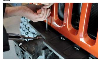
6. Remove the two bolts that hold the vacuum pump into the mount on the Jeep's frame.
