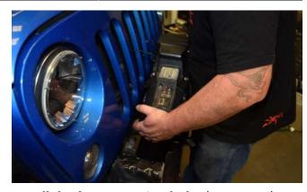
**25. Install the four mounting bolts** that came with your winch, through the bottom of the Recessed Winch Cradle, into the mounting nuts in the winch.
