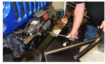
**32. With the help of a** friend, lift the bumper/skid assembly into position on the Jeep.
