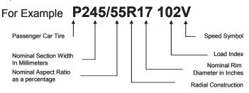
**Speed Symbol:** an alphabetic code indicating the maximum speed at which the tire can carry a load corresponding to its Load Index under specified service conditions.
