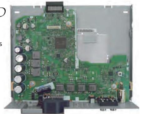
Large Capacitor and Plate-Type Heatsink
