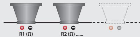
$$R1 (\Omega) + R2 (\Omega) + \dots + Rn (\Omega) = Rt (\Omega)$$
