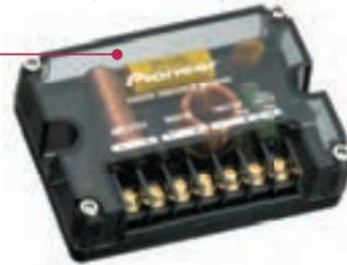
Large air core coil eliminates signal transmission loss.
