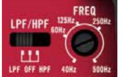
Variable LPF and HPF allow for adjustable frequency between 40 Hz to 500 Hz\* and greater car audio system flexibility according to subwoofer characteristics and personal listening preference.
