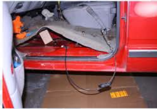
E.) Pull carpet up as high as possible. Remove floor grommet and pull cable out.
