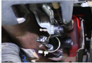
F.) Tilt steering wheel to upper position. Place shifter in 1st gear position. Use wide blade screwdriver to pop off end of shift cable.
