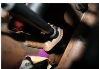
G.) Use screwdriver to release tabs at mounting bracket (on steering column) under dash.
