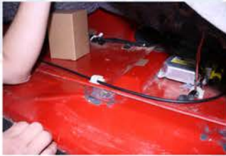
E.) Pull carpet up as high as possible. Remove floor grommet and pull cable out.
