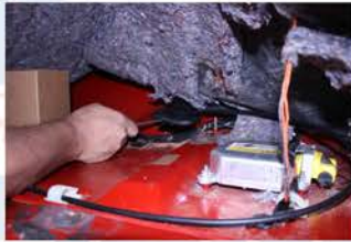
E.) Pull carpet up as high as possible. Remove floor grommet and pull cable out.
