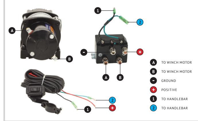
Use the diagram below to set up your PS6000, PS9000, PS120000, or PS20000 winch wiring.
