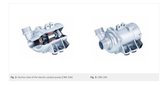
The electronics in the motor casing were developed inhouse. They measure the rotor position of the motor without a sensor and provide current – depending on its position – to the stator windings. Regulation of the electric coolant pump takes place via the hybrid-designed electronics, which receive relevant information from the motor management system and use it to set the flow of coolant needed in each case. Both PWM signals and digital signals like the LIN-bus can be used for this.
