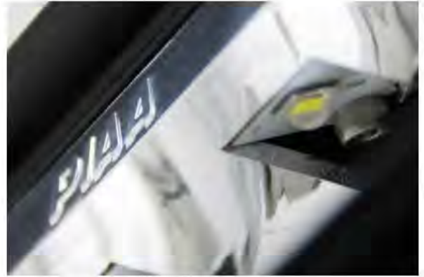
REFLECTOR FACING LEDs
