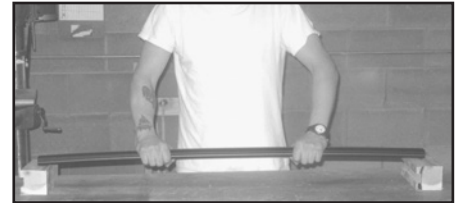
Decrease Rail Curvature-Rail Right Side Up
