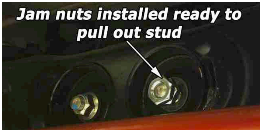
Shows nut removed, and jam nuts installed ready to remove stud from diff cover.
