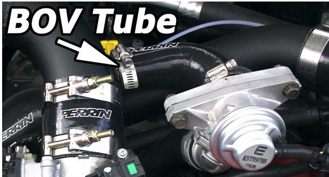
OEM BOV Being Connected to FMIC boost tube. Note there is no kink in BOV tube.
