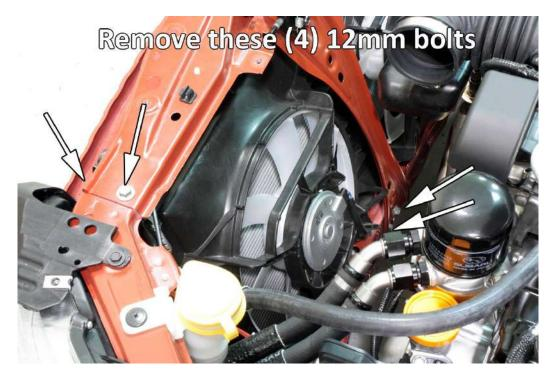
8. Lift up on left side of radiator support (leaving intake air diverter in place) and place PERRIN intake tube under support as shown below. Make sure that tab on PERRIN intake is in front of radiator support and closely lines up to threaded M6 hole shown below. Carefully set radiator support back down and reinstall (4) 12mm bolts removed earlier.
