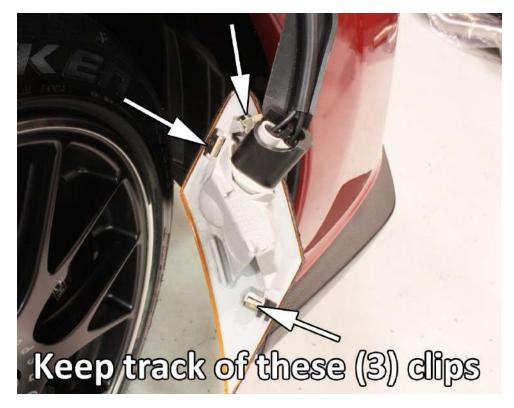
e. Behind each side marker is a single plastic fasten that needs to be removed. This fastener is a little tricky and may require a pick tool and or a bent awl.
