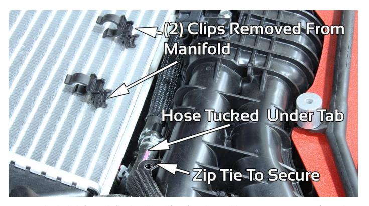
11. Set shroud on back of intercooler first, then pull toward front of car to line up with large spacers. Foam tape at rear of intercooler is designed to compress when installed and also designed to work with aftermarket intercoolers.
