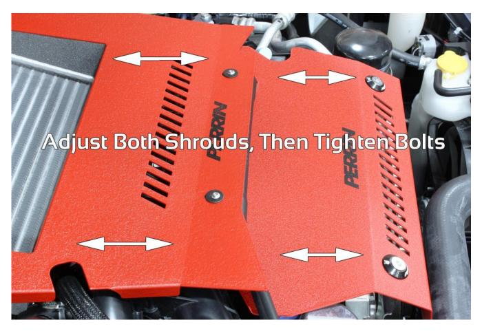
14. Adjust plastic hose, intercooler shroud and belt cover until it is lined up with front of car. Tighten 10-32 screws until hand tight.
