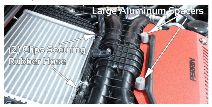
10. Tuck rubber hose under plastic tab as shown below. Secure with supplied zip tie. This is important to add clearance to the intercooler shroud being installed.
