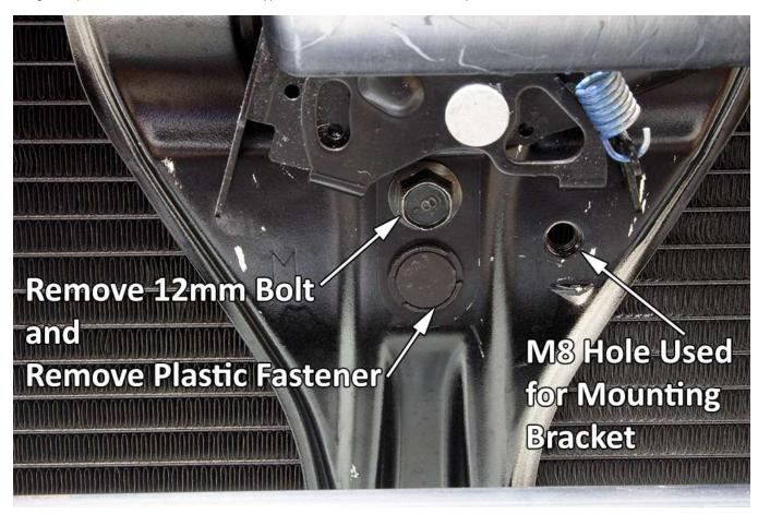
3) Locate and remove OEM horn on lower radiator core support. You will re-use 12mm bolt (not the nut) in future steps.
