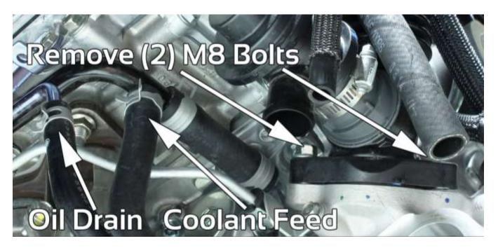
11. Removed (2) M8 bolts securing plastic boost tube to turbocharger (shown above). Note: Rear most bolt is difficult to reach and best to use a gear wrench to remove.
