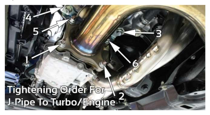
27. Loosen (2) M8 bolts securing upper turbo support bracket at engine, then re-tighten to 15ft-lbs. **NOTE: This step is important to relieve** any unwanted pressure on the PERRIN header. In the same order as in the above step, fully tighten bolts and nuts to 31ft-lbs. **NOTE: Not** using the OEM turbo/header support brackets will cause the header to fail and will void the warranty on your PERRIN Header.
