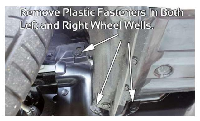
3. Using proper panel removal tool or flat head screw driver, locate and remove (7) plastic fasteners and (2) 12mm headed bolts from lower portion of splash guard. See picture below.
