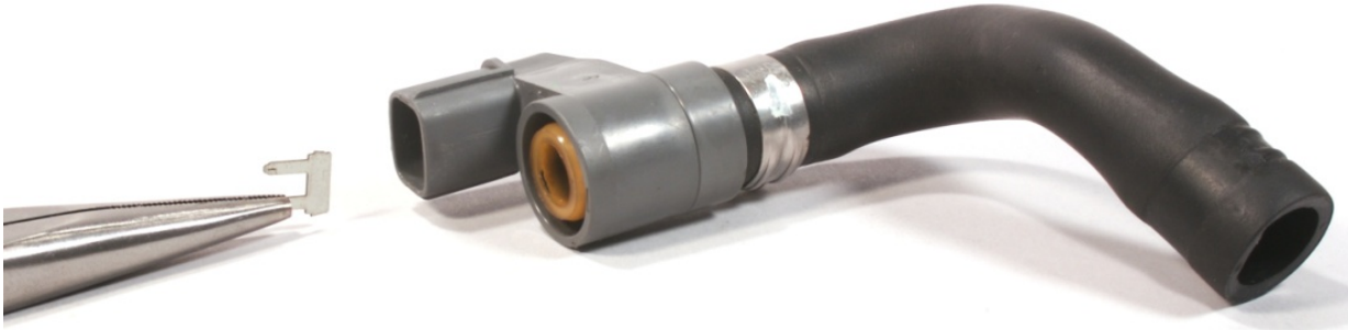
Pin shown being removed from PCV diagnosis connector
