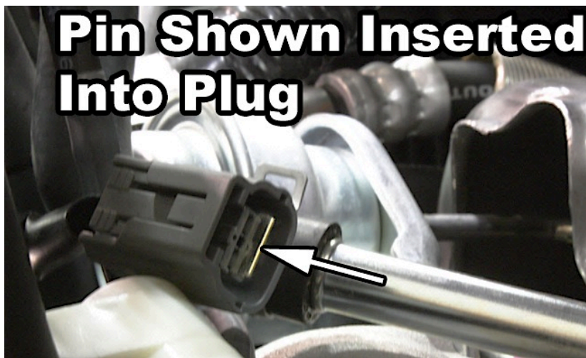
Pin shown inserted into PCV diagnosis harness.
