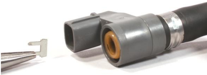
Above diagrams show pin being removed from PCV diagnosis connector and the connector with female pins to reinstall it to.
