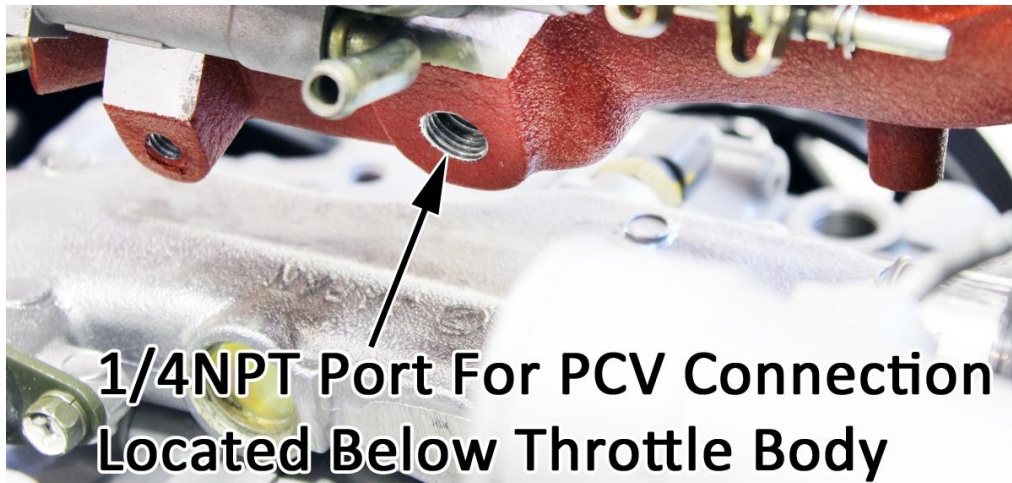
Above picture shows 2002-07 WRX/04+ STI manifold port for PCV connection. Shown with fitting (or PCV on 02-03 WRX) removed.
