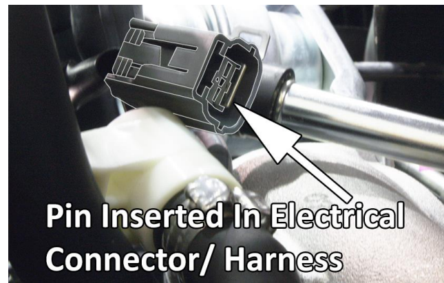
Above diagrams show pin being removed from PCV diagnosis connector and the connector with female pins to reinstall it to.
