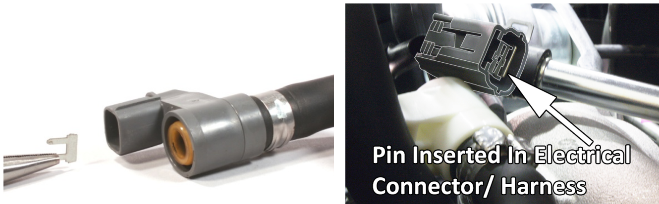
Above diagrams show pin being removed from PCV diagnosis connector and the connector with female pins to reinstall it to.
