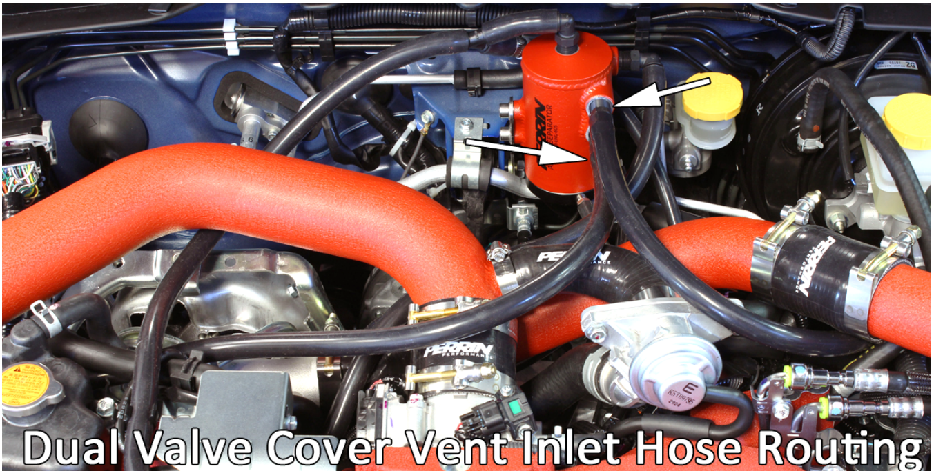
Above diagram shows 04+ STI using both valve cover vent inlets on AOS body.
