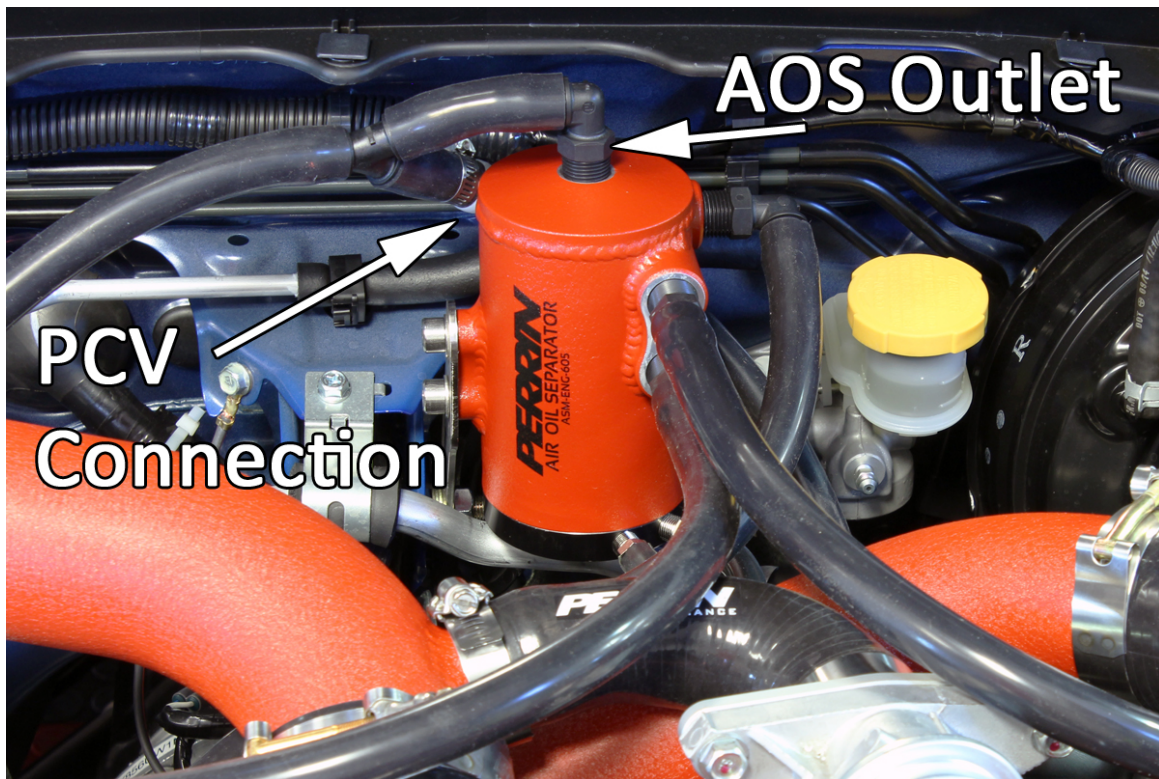
Above diagram shows 04-07 WRX and 04-13 STI setup. 02-03 WRX will NOT have PCV valve located as shown.
