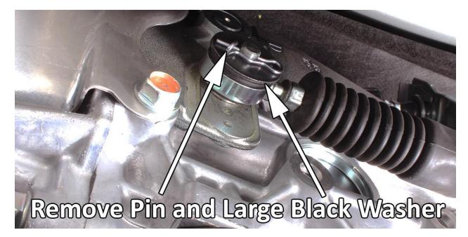
Locate pin securing shift cable and bushing to pivot on shift linkage. Remove pin and large black washer behind it.
