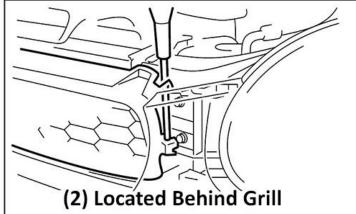
b. For 06-07 cars, on center grill, remove (2) small plastic fasteners from top section. Carefully pull grill straight out from bumper to expose mounting location. There are 4 large clips holding this in place and they can be kind of tight while removing.
