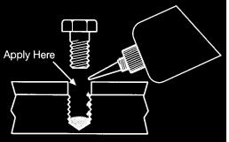
Assemble and tighten as usual. When tightening to established torque values, torque compensation is not required.
