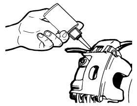
Any excess grease that squeezes out from the mating surfaces should be removed. Note: Keep lubricant off pads and rotors.
