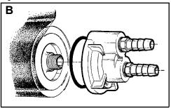
Install the threaded nipple into the bottom of the remote oil filter mount. Insert the shortest end in the mount and tighten securely. Repeat for dual mount, if applicable. (Illustration C). DO NOT use Teflon tape on filter nipple.
