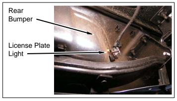
**j.** Install rear bumper wiring harness onto frame, if possible.
