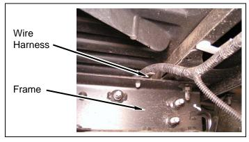
**k.** Install *kit* **tie** (zip) onto rear crossmember and bumper wiring harness.
