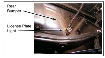
Remove four bolts and rear bumper from O.E. trailer hitch brackets.
