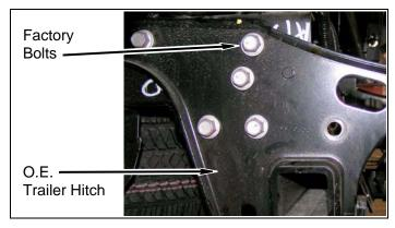
e. Apply a small amount of kit Loctite® onto threads of eight factory bolts and install rear bumper and kit brackets (rear bumper) onto O.E. trailer hitch with eight factory bolts. DO NOT TIGHTEN.
