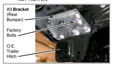
f. Install two *kit* brackets (rear bumper) onto O.E. trailer hitch with two *kit* bolts (9/16" x 1-1/2"), four *kit* washers (9/16" SAE), and two *kit* nuts (9/16" stover). DO NOT TIGHTEN.
