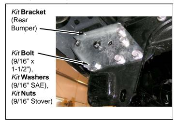
g. Install kit bracket (rear bumper, middle) onto rear bumper with two factory bolts and nuts. DO NOT TIGHTEN.
