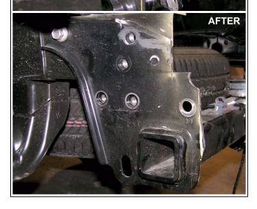
b. Apply a small amount of kit Loctite® onto threads of two factory bolts and install kit bracket (rear bumper, passenger) onto passenger side bumper with two factory bolts. DO NOT TIGHTEN.
