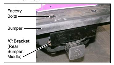
h. Install kit bracket (rear bumper, middle) onto O.E. trailer hitch with two kit bolts (1/2" x 1"), four kit washers (1/2" SAE), and two kit nuts (1/2" stover). DO NOT TIGHTEN.
