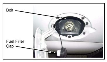
c. **2005 model:** Remove bolt and fuel filler from frame.
