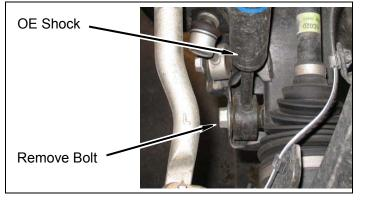
c. Remove two bolts and lower ball joint from knuckle.
