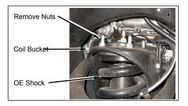
f. Pry lower control arm downward and remove strut from vehicle.
