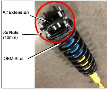
**b.** Reinstall the strut assembly in its stock location. Leave the four upper strut mounting nuts loose.
