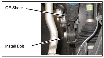
**d.** Use a floor jack to raise the lower control arm up in order to get the two lower ball joint bolts installed. TORQUE bolts to OE specification.
