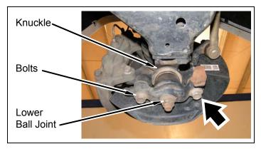
d. Loosen lower control arm cam bolts to release tention from bushing and allow lower arm to droop down when disconnected from lower ball joint mount.
