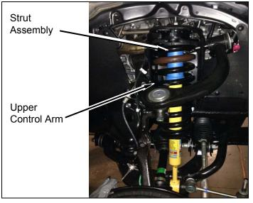
**c.** Raise the lower control arm and install strut assembly onto lower control arm with OEM nut and bolt. DO NOT TIGHTEN.
