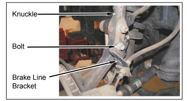
**h.** Install sway bar end link onto knuckle with nut. TORQUE nut to OE specification.
