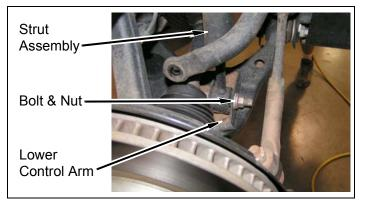
**d.** Use a floor jack to raise the lower control arm up in order to get the two lower ball joint bolts installed. TORQUE bolts to OE specification.
