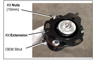
**b.** Reinstall the strut assembly in its stock location. Leave the three upper strut mounting nuts loose.
