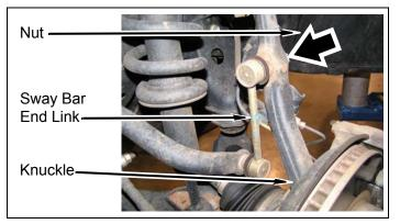
**b.** Remove bolt and brake line bracket from knuckle.
