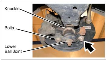
f. Remove strut assembly from vehicle.
