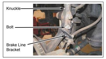
**c.** Remove lower nut and bolt from lower control arm and strut assembly.
