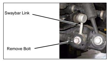
b. Remove lower shock bolt.
