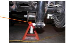
38. Disconnect the lower sway bar end link nut with a 16mm wrench.
