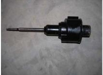
28. Install the boot over the strut and with one of the replacement washers, pull the boot over the washer at the top of the strut and zip tie the boot to the bottom of strut.
