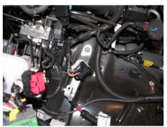
12. Remove the axle vent tube and ground wire from the 2 strut studs.
