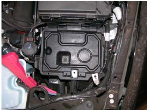
5. Disconnect the power lead (2) to the totally integrated power module (TIPM 3) by opening the cover (4) and remove the nut with a 11mm socket (1).
