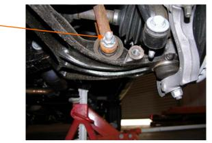
20. Remove the upper control arm ball joint nut with a 21mm wrench and separate the upper ball joint from the knuckle.
