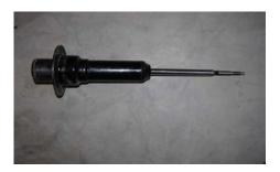
27. Install the spring spacer onto the strut, note the location of the spacer bump stop on the side of the spacer, as it needs to face out ward on the strut. There is a notch on the spacer that will match a locator on the strut.
