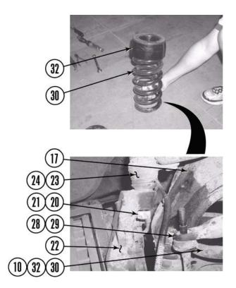
e. Install sway bar (29) on sway bar link (28) with bushing (27), washer (26), and nut (25). Torque nut to 27 ft-lbs.
