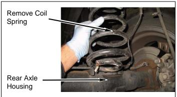
8. Removing rear coil spring Isolator from both coil spring.
