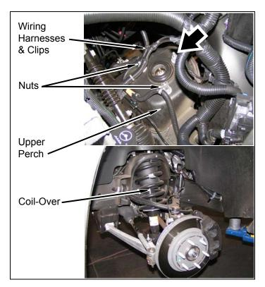
Remove two lower coil-over bolts from lower control arm.
