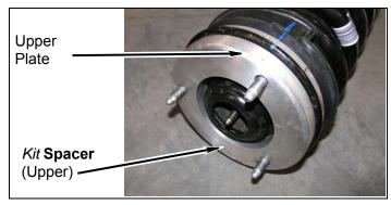
b. **From CL230BAG:** Install coil-over onto upper perch with three *kit* **washers** (10mm) and three *kit* **nuts** (10mm stover) and *kit* **Loctite**®. TORQUE to OE specification.
