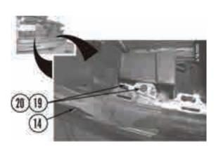
e. Remove four pull clips (21) and air scoop (22) from core support (9).
