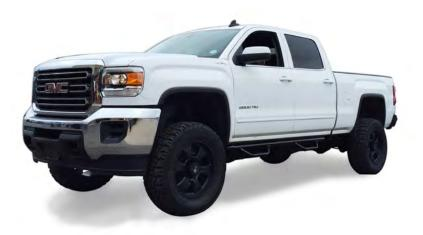
Performance Accessories Body Lift raises your vehicle's body 3" over the factory frame, allowing the use of up to 33" diameter tires. Installation maintains OEM <u>suspension</u> geometry and improves on and off-road capabilities.
