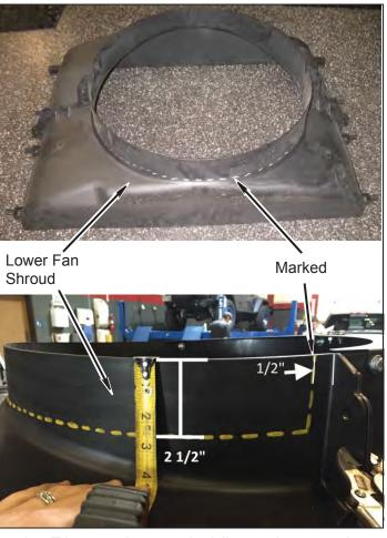
b. Trim cut along marked line and remove lower section of lower fan shroud.
