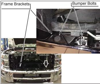
e. Install two kit sleeves (bumper, front, support) onto bumper with two kit bolts (M10-1.5 x 100mm) between bumper and OEM side support bracket. DO NOT TIGHTEN
