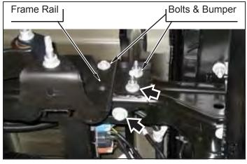
Remove two bolts and bumper from hitch and vehicle.
