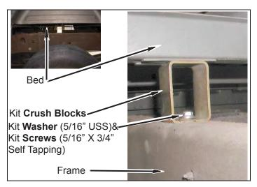
5. Finish the bed kit lift block installation.
