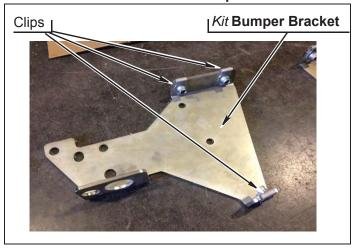
**f.** Position two *kit* **brackets** (bumper, rear) onto bumper and reinstall OE bolts.
