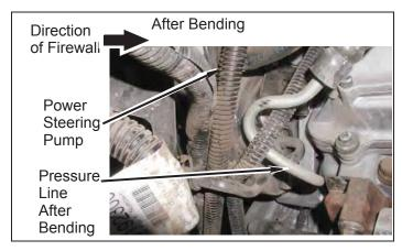
d. Carefully bend power assist pressure line up toward hood, to clear accumulator on brake hydro boost.
