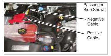
b. Install kit extension bracket (L-bent) using OEM nut onto battery terminal fuse junction and kit hardware (5/16") at positive cable end as shown below:
