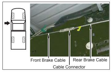
d. Remove front brake cable and brake cable housing from front frame mounting pad.
