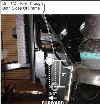
**b.** Install OEM 12mm bolt through newly drilled hole and tow hook.
