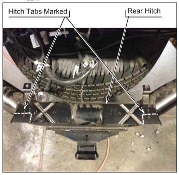
k. OEM Hitch Tabs Removed.
