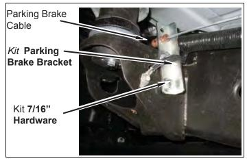
c. Install two ground wires onto kit parking brake bracket with kit bolt (1/4") nut and washers. Connect front and rear brake cables. Remove clamps from rear cable.
