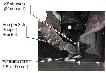
f. Adjust bumper to body clearance using measurements from removal section. Align bumper to previous measurements and TIGHTEN all bumper hardware.
