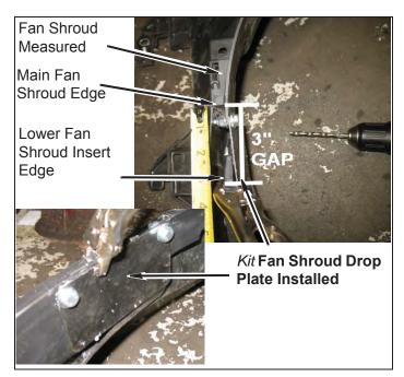
f. Once you have shaped and placed each kit fan shroud drop plates into place; re-clamp and secure each kit shroud plate at a 3" gap and mark each 1/4" holes for drilling.
