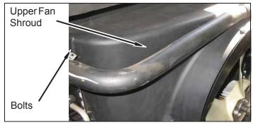
b. Remove six pop-ups and upper fan shroud from vehicle.
