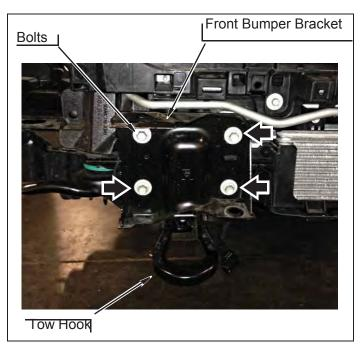
f. Remove four bolts, two nuts and two tow hooks from frame horns.
