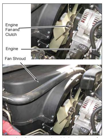
o. Install two upper shroud bolts onto upper fan shroud and core support.
