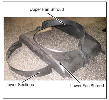
c. Assemble fan shroud using six OEM push clips.
