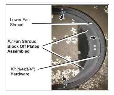
m. Install *kit* **lower fan shroud block off plate anchor** onto *kit* **lower fan shroud block off plate** assembly by using existing *kit* (1/4") hardware and drilling a 1/4" hole into center of the shroud and installing *kit* (1/4") hardware to anchor center of lower shroud assembly.
