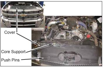
b. Remove four bolts from top of grille and disconnect lower grille clips from core support to remove grille.
