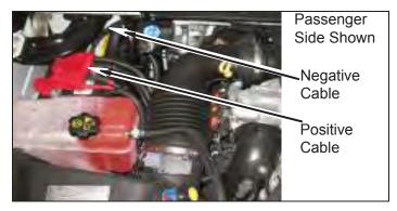
b. Disconnect positive starter cable from battery junction as shown in image:
