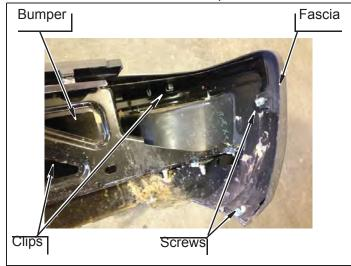
**c.** Remove plastic fascia from corner of bumper by gently using a pry bar to loosen each clip.
