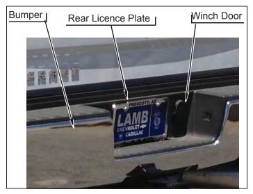
**b.** Remove three clips and two screws from each inside fascia and rear bumper.
