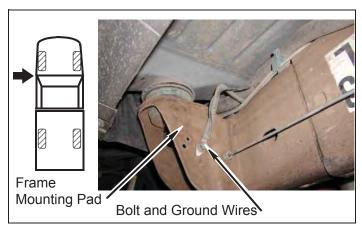
Pull some slack in parking brake cable. Clamp two cables at cable housing where indicated by arrows.
