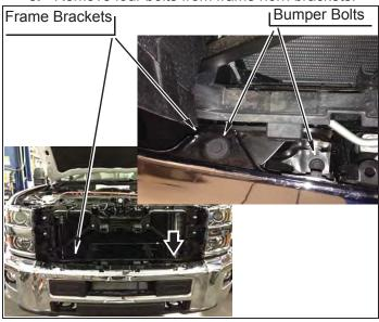
**d.** Remove front bumper from frame horns.
