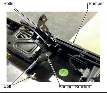
**e.** Remove u-nuts from OE Bumper bracket and reinstall u-nuts onto *kit* **bumper brackets**.
