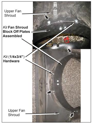
I. Using second pair of kit fan shroud block of plates. (Leave brackets slightly loose until mounted onto fan shroud, this will allow you to adjust the plates as needed to fit shroud properly.) With both kit fan shroud block off plates assembled, face the tabs outwards so that the kit fan shroud block off plate assembly mounts evenly with the inside edge of the lower fan shroud assembly. (Tighten assembly now.)
