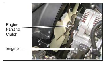
d. .Remove lower fan shroud from clips.
