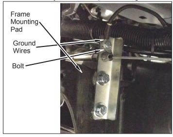
d. Remove dvr side wiring harness from frame rail and secure it to fuel and brake lines using *kit* **zip ties**.
