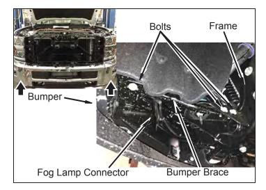
c. Remove four bolts from frame horn brackets.
