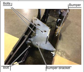
**g.** Use two *kit* **thick washers** in-between *kit* **bumper bracket** and bumper corner support bracket before installing both OE center bolts.
