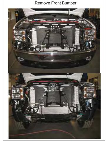
e. Remove eight bolts from front frame horn brackets and remove both front bumper brackets from frame horns.
