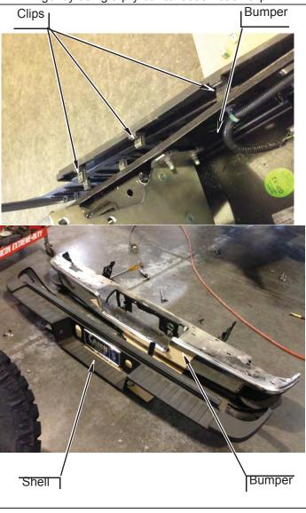
**d.** Remove five torx bolts from each bumper bracket and remove bumper bracket from shell.
