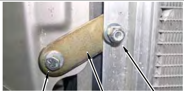
Kit Bolt, Washers, and Nut Kit Drop Down Bracket Kit Washer and Nut
