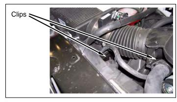
e. Remove engine air intake hose.
