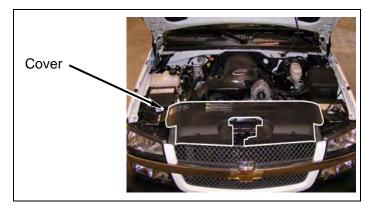
Remove six clips and grill from core support and front fenders.
