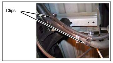
k. Install ground wire to frame rail with factory bolt.
