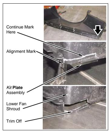
i. Position lower fan shroud and kit plate assembly together as marked. Using kit plate assembly as a template, drill five 1/4" holes.
