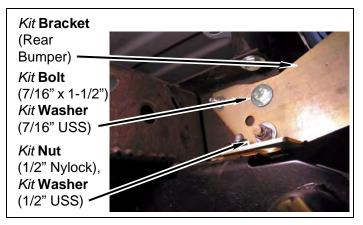
2" kit: Install kit brackets (rear bumper, 1-stud) with four kit bolts (7/16" x 1-1/2"), eight kit washers (7/16" USS) and four kit nuts (7/16" Nylock). DO NOT TIGHTEN.
