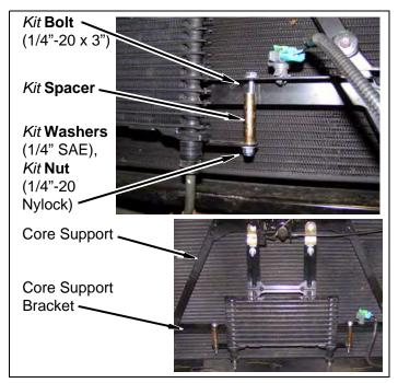
e. Adjust transmission cooler and position transmission cooler lines in factory clips.
