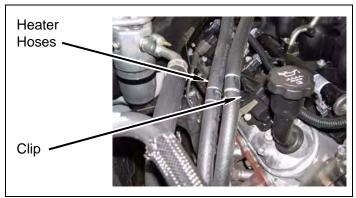
h. Install wiring harness into wire clip.
