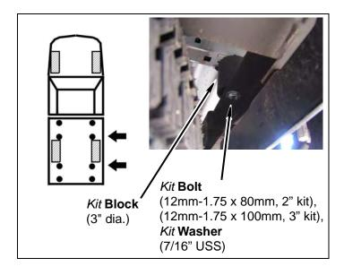
d. Place a *kit* **block** (2" diameter) on rear bed frame mount.
