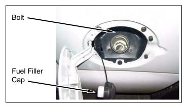
i. Install fuel filler to fuel filler hose. Adjust kit extension (fuel filler, rubber) and fuel filler hose.
