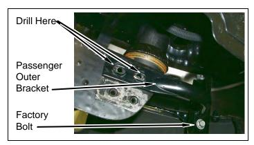
j. 2" kit: Install passenger side outer bracket to frame with two kit bolts (7/16" x 1-1/2"), four kit washers (7/16" USS) and two kit nuts (7/16" Nylock). DO NOT TIGHTEN.
