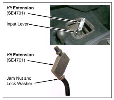
b. Install shift lever on *kit* extension. Tighten jam nut.
