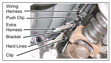
c. Remove two nuts and bracket from transfer case.
