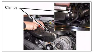
d. Disconnect overflow and radiator hose from clips.
