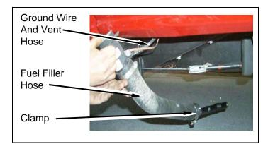
Carefully cut filler hose in half as shown. DO NOT CUT THROUGH PLASTIC TUBE INSIDE FILLER HOSE.
