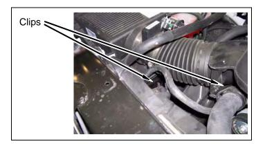
c. Tighten engine air intake hose clamps.
