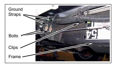
d. Remove wire clips from body and frame rail along passenger side.
